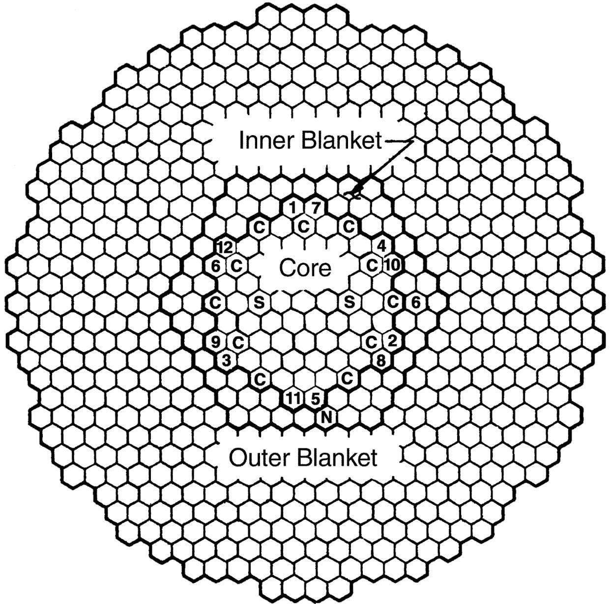
Figure 7. Full core layout of EBR-II [26].
