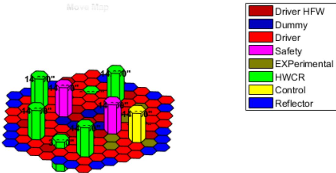
*Figure 17. Control rods in the critical configuration.*
