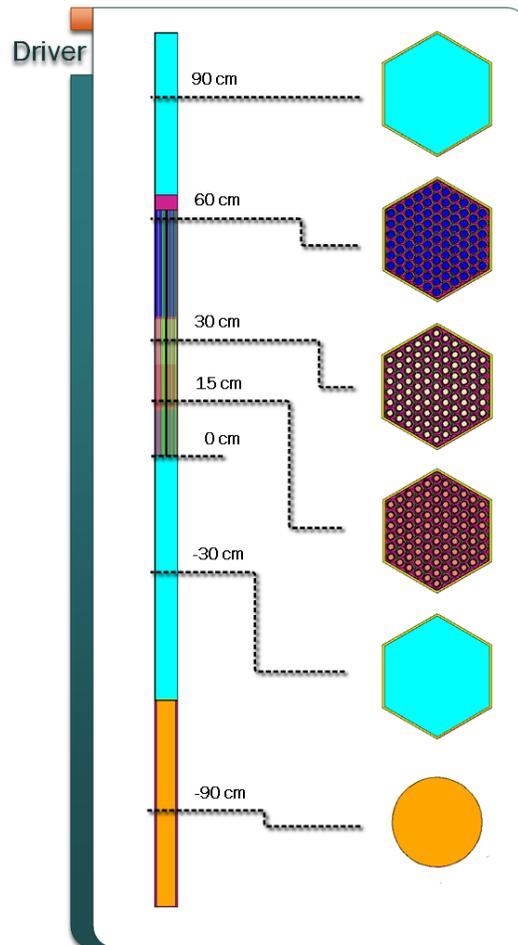
Figure 8. MCNP plot of driver subassembly [26].
