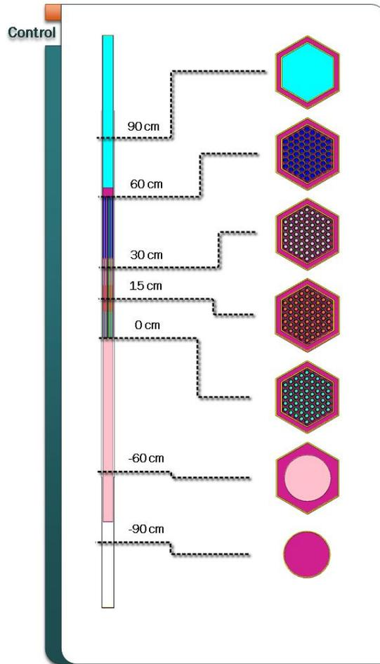
Figure 16. MCNP plot of the control subassembly [26].
