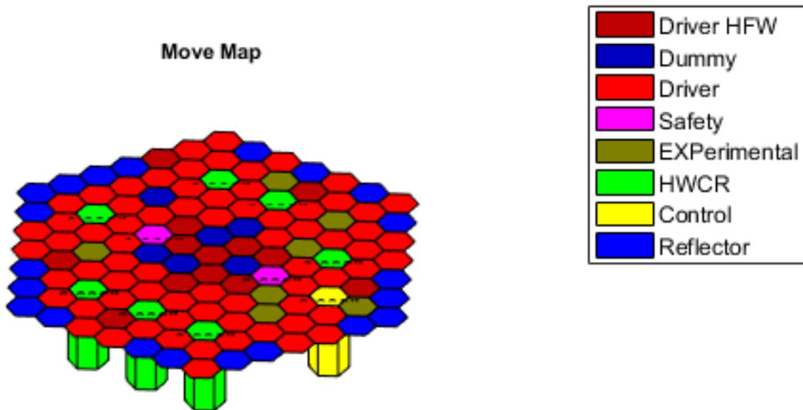
*Figure 18. Control rods in the subcritical configuration.*
