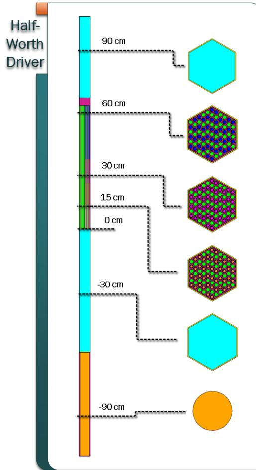
Figure 9. MCNP plot of half-worth driver subassembly [26].
