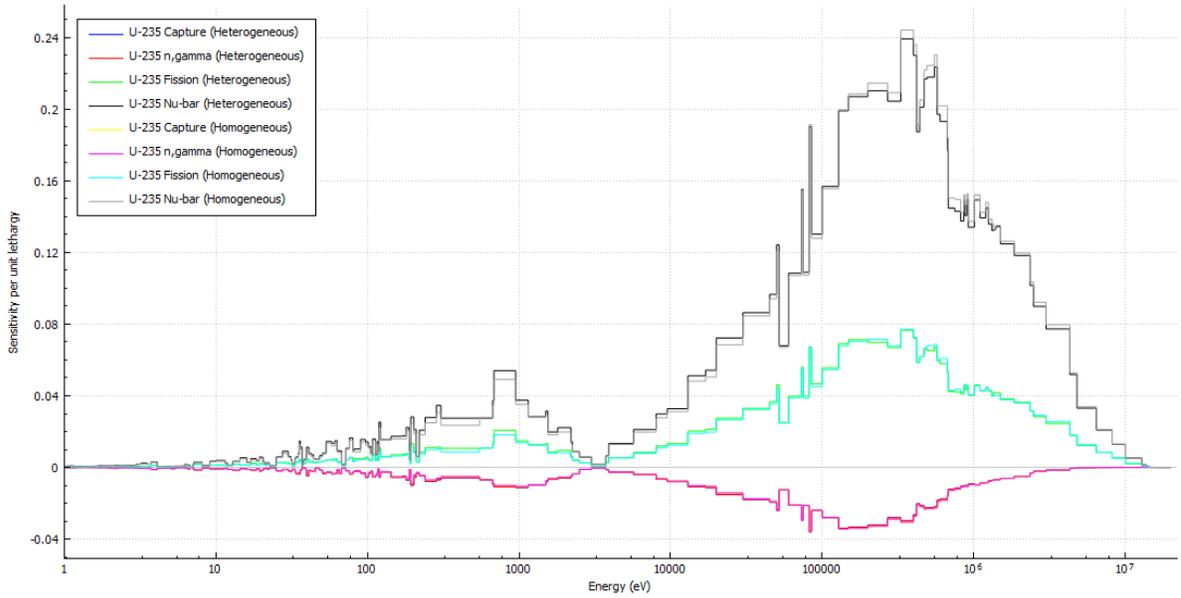
*Figure 28. The energy, region, and mixture integrated sensitivity coefficient plot for the uranium-235 cross-sections for the heterogeneous and homogeneous model.*
