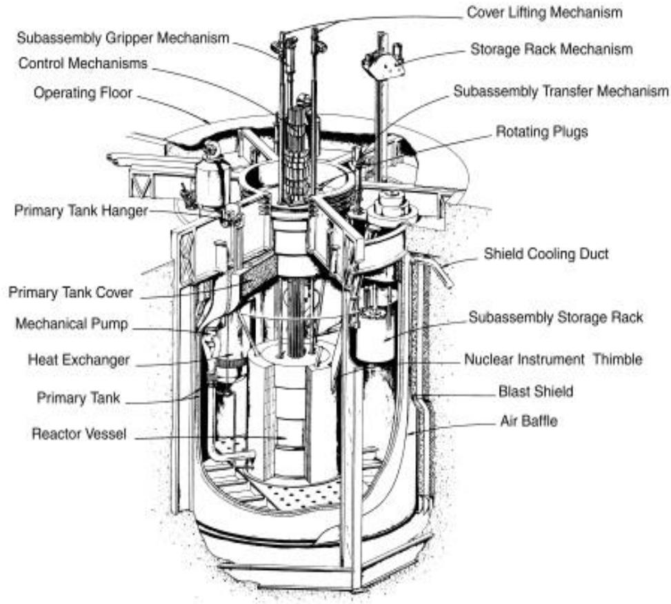
Figure 4. Detailed layout of the primary coolant system [4].
