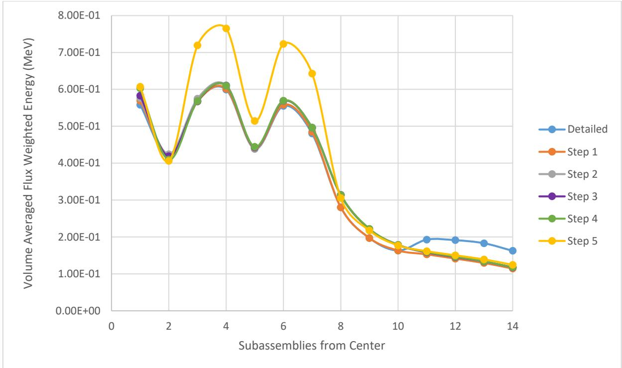
Figure 23. Volume averaged flux weighted energy vs. distance from EBR-II center.
