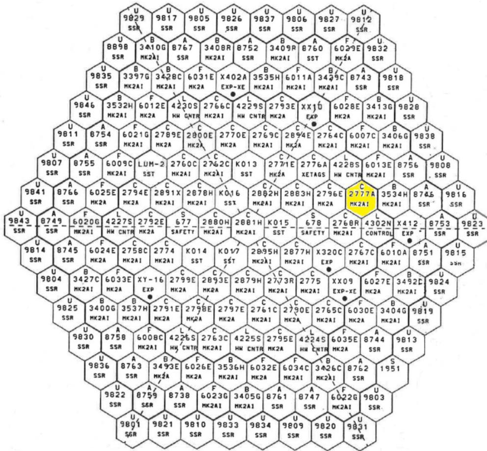
Figure 6. Core layout and the subassembly position scheme [25].
