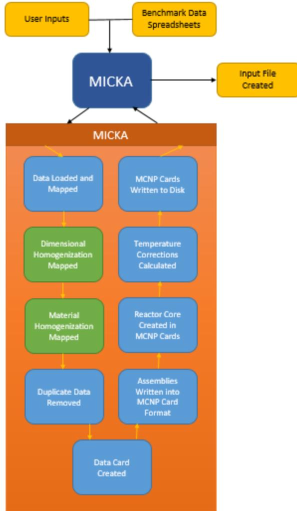
Figure 22. MICKA flow chart with homogenization function additions.
