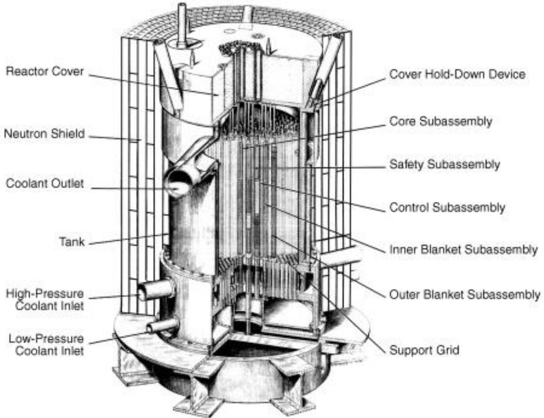
Figure 5. Design layout of the EBR-II core [4].
