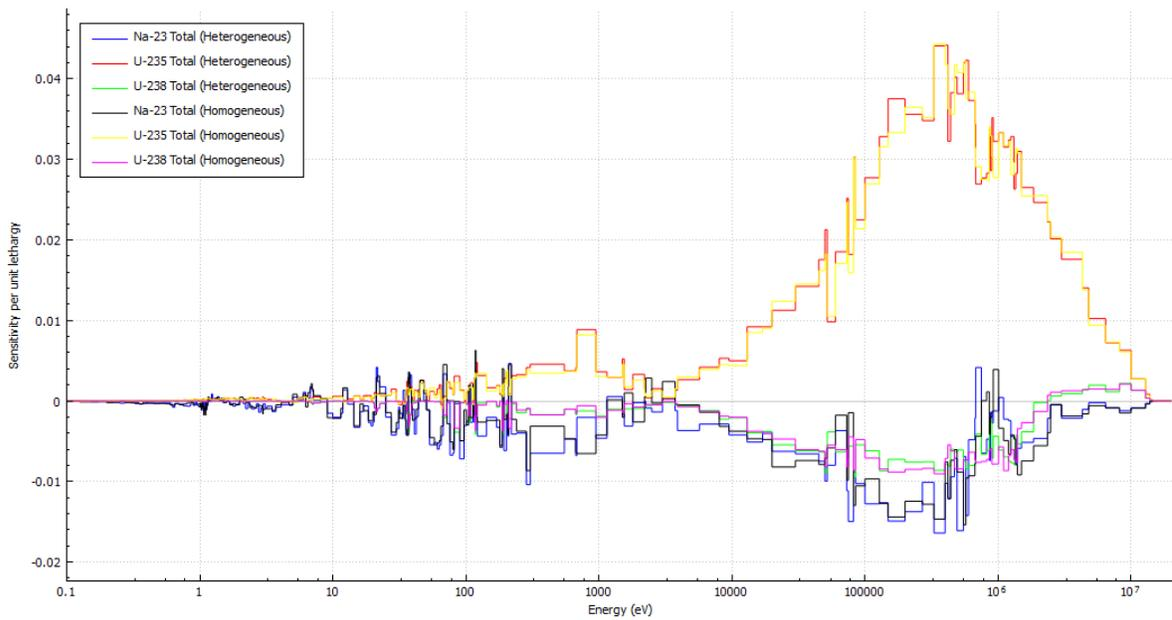
Figure 27. The energy, region, and mixture integrated sensitivity coefficient plot for the total cross-sections for the heterogeneous and homogeneous model.
