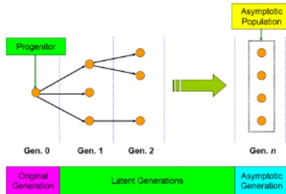
Figure 2. The iterative fission probability method [18].
