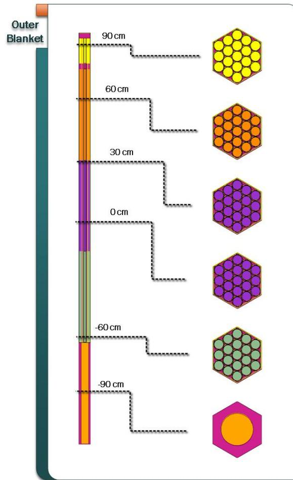
Figure 12. MCNP plot of blanket subassembly [26].
